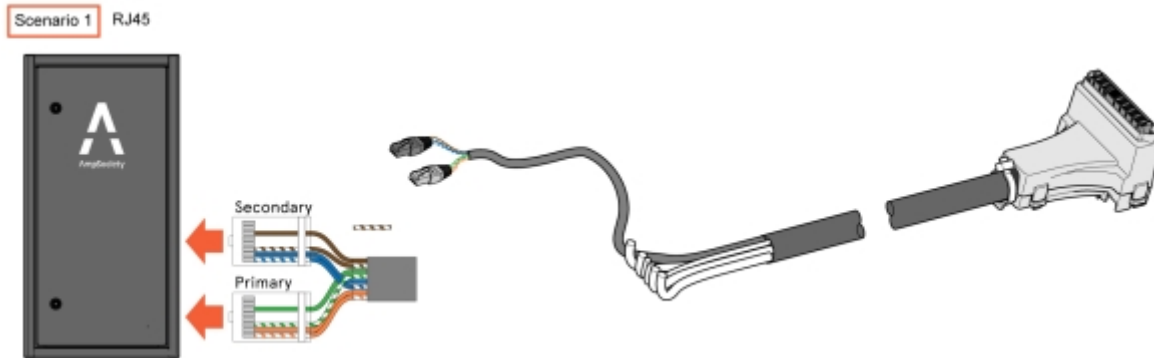
Image 63: Connection between SmartHub and one ConnectCable
