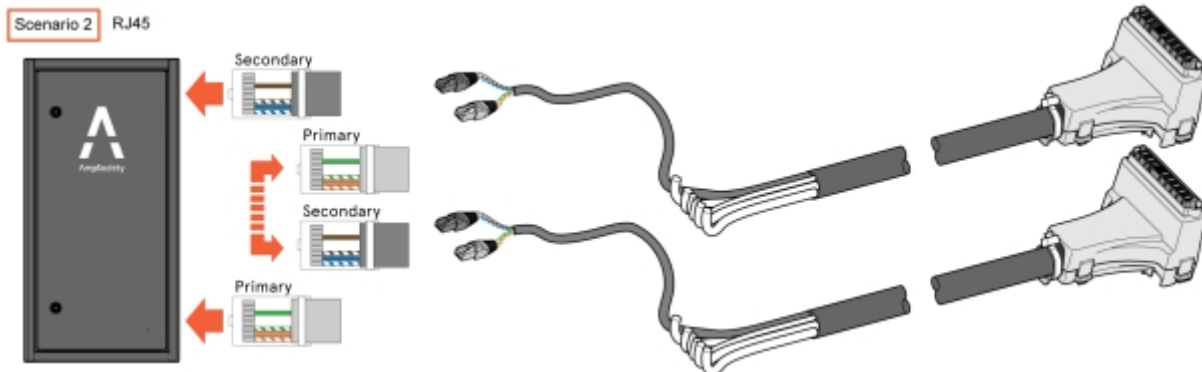
Image 64: Connection between SmartHub and 2x ConnectCable
